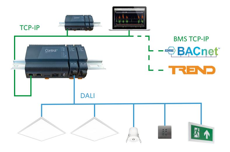
Control<sup>3</sup> processors are connected with a standard TCP-IP ethernet network. Any laptop or PC on the network can access the web based user interface for control and configuration.
