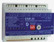
SAM-24 Remote circuit monitoring unit for 8 lighting circuits with RS485 comms.
