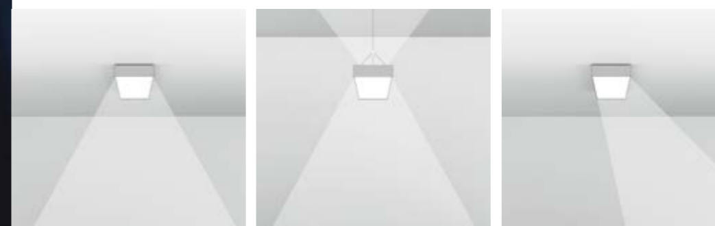
Light distribution in direct, direct-indirect and asymmetrical distribution versions
